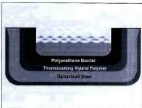
TriArmor® Corrosion Protection System Triple Layer Protection of the Cold Water Basin
