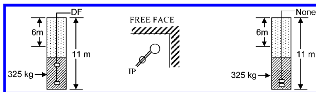
1 Blast design layout with charging pattern for signature blast detonated by DF and Nonel initiation system at Jayant project
