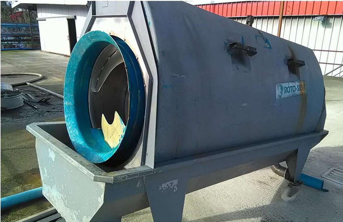
Figura 11: Rotofiltro Rotosieve
