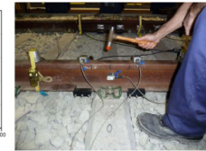
Figure 5-45: Static test wheelset loading protocol (left) and set of accelerometers used in the receptance tests (right).
