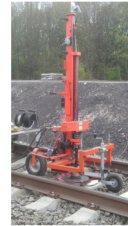
Figure 4-3: Hydraulic driven drop weight "DYNPACT" as an example for falling mass as used within RIVAS project WP 1 and WP 3 (picture Detusche Bahn AG R. Garburg)
