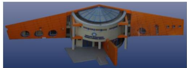
Figure 13. 3D model of a building generated from Unmanned Aerial System (Oniga, Chirilă, & Stătescu, 2017)
